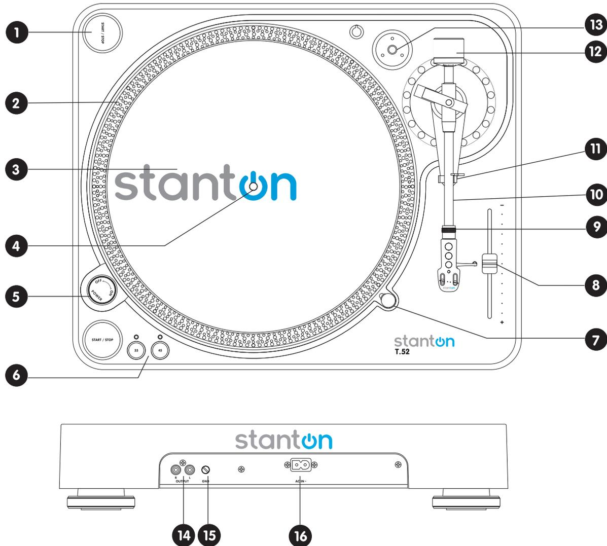
**1. Start/Stop** - Press this button to start or stop the platter.
