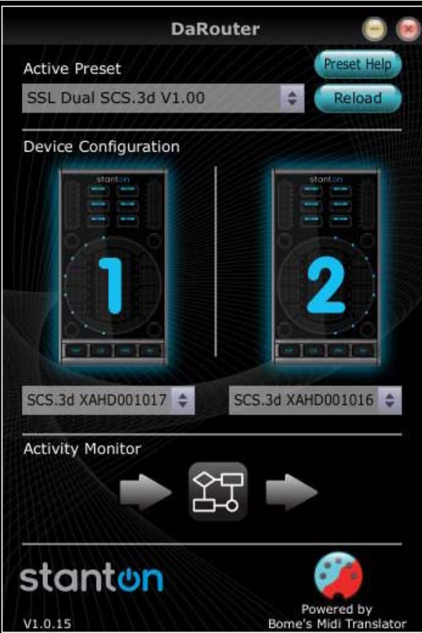
Proper DaRouter configuration, preset selected and units are lit blue to indicate connection
